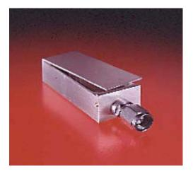
**DESCRIPTION** The Microphase Highpass Filter will pass all frequencies from 20 MHz to 2000 MHz and block all frequencies below 15 MHz by -60 dB. The Highpass Filter has uses in many types of military applications including: RF communication and navigation systems.
