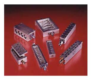
**DESCRIPTION** The Microphase Bandpass Filters offer five different design types which have a range of capabilities and options. These filters have a passband frequency of 500 MHz to 40 GHz and bandwidths of up to one octave. They maintain rejection levels to 90 dB, VSWR from 1.2:1 to 2.0:1 and an Insertion Loss as low as 0.35 dB.
