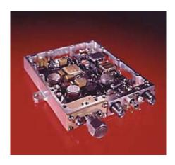
**DESCRIPTION** The Microphase 62 dB Dynamic Range, DC-Coupled DLVA serve an essential function in modern radar and electronic warfare systems. This logarithmic amplifier compresses a much larger input dynamic range into a small output dynamic range. The most common applications within radar and EW systems are direction finding and power monitoring
