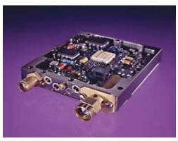
**DESCRIPTION** The Microphase High Speed DC Coupled DLVA DFH Series A serve an essential function in modern radar and electronic warfare systems, This logarithmic amplifier compresses a much larger input dynamic range into a small output dynamic range. The most common application within radar and EW systems are direction finding and power monitoring.
