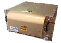
Shown at left is an air to water cooling system used onboard US Navy submarines. This compact heat exchanger cools 6kW of electronics through the chilled water system provided by the boat. Units are designed for handling high shock, vibration and other tough environmental requirements in the smallest form factor possible. AMETEK Rotron can also provide superbalanced assemblies to conform to some of the most rigorous structureborne noise requirements typically found on submarines.
