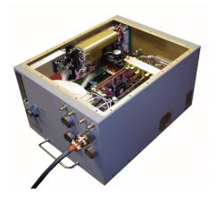
The photo on the left shows a typical chassis that this type of system is installed in. The cooling unit is integrated into the bottom 3.5" of the chassis. Cold air is circulated through the electronics. The heat is then exhausted to the atmosphere thru the holes shown on the side the chassis.
