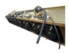
The system shown at the left is another example of a radar cooling system. The eight cooling fans and two scavenge fans are all controlled by a common fan controller that can vary the speed to the fans based on temperature inputs. The use of high speed AMETEK Rotron vaneaxial fans allows the customer to achieve extremely efficient cooling in a very small package.
