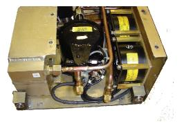
The system shown on the left is an active refrigerant (R134A) based cooling system. The system cools an electronics chassis on an Military aircraft.
